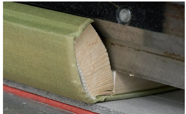
Figure 4: A test with cut & scan digitization at the KB – on a lot of second-hand books (Photo: Jos Uljee, KB)
